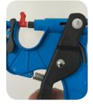
**2c.** Carefully squeeze the plier handles until the large piston comes to a stop against the red connection piece
